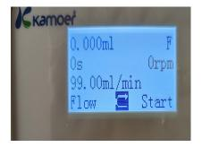
Press Enter while flow is selected. Set the flow speed to 80.00ml/min. flow speed can be adjusted as needed. Follow the instructions in the pump manual to adjust flow rates.
