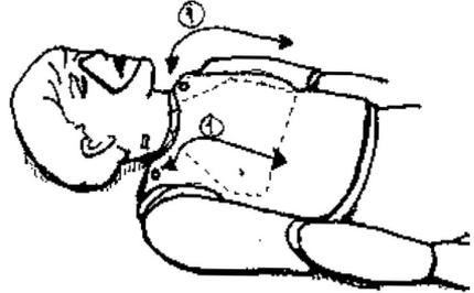
2. Remove the head from the manikin by pulling the retaining pin straight back from the rear of the manikin neck.
